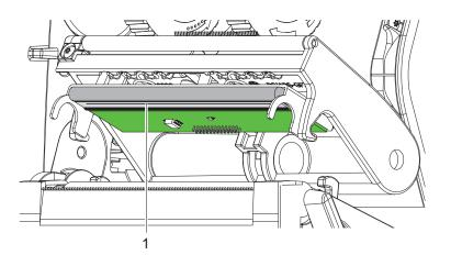
Figure 16 Heating line of the printhead
