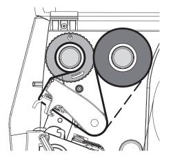
Figure 13 Transfer Ribbon Feed Path
