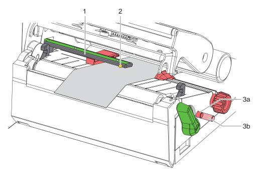
Figure 10 Adjusting the label sensor
